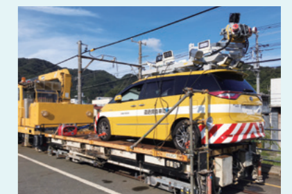
Vehicle measuring 3D point group data
