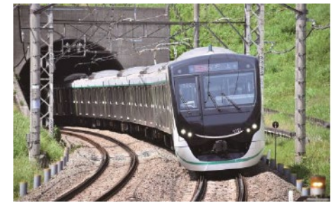
The 2020 series trains that have reduced electricity consumption by 50% compared with the previous models
