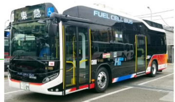
The SORA fuel cell bus which uses hydrogen as its fuel
